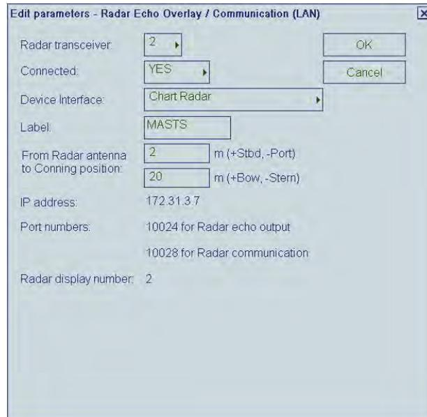
**Note 1:** "Radar display number" defines IP address for connected ARPA Radar Display.
