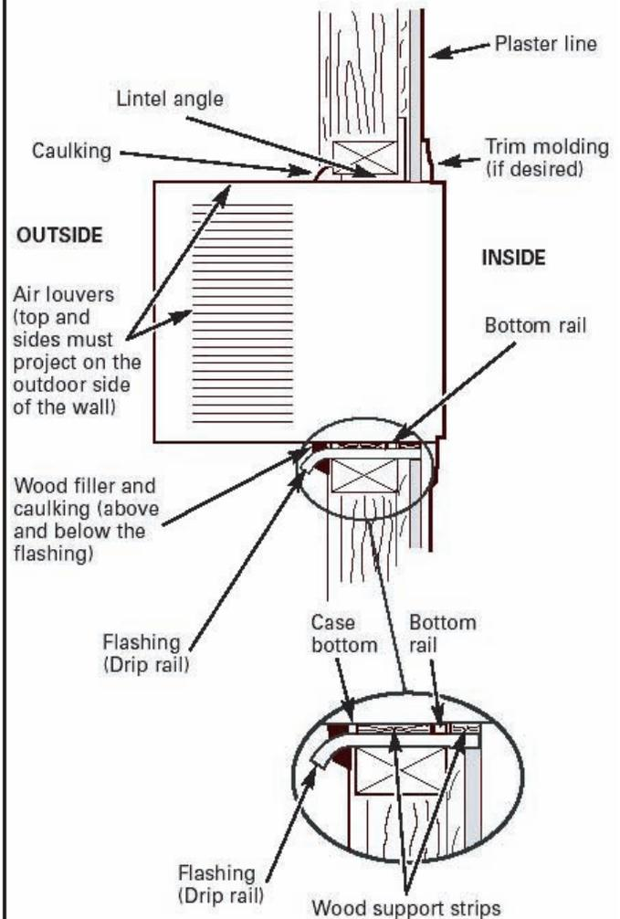
**B** Place the air conditioner into the case. For specific instruction, refer to the Window Installation Instructions.
