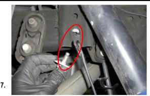
Remove the 13mm emergency brake line support bracket on the passenger side frame rail.
