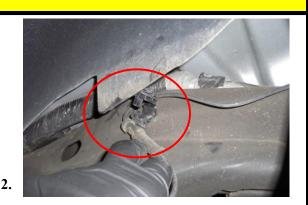
Unhook the ABS line at the frame on the both sides.
