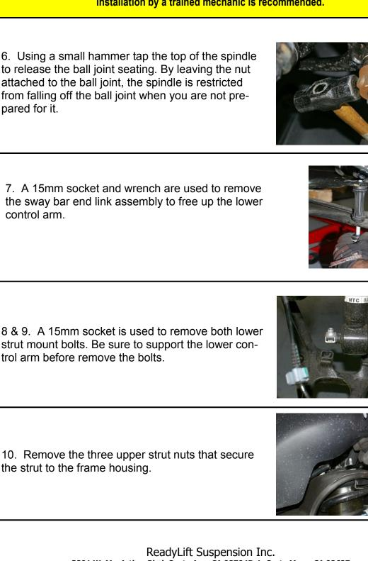
6. Using a small hammer tap the top of the spindle to release the ball joint seating. By leaving the nut attached to the ball joint, the spindle is restricted
