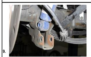
Remove the 21mm lower shock mount bolt on both sides.
