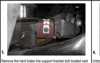
to the lower track bar mount on the driver side.
