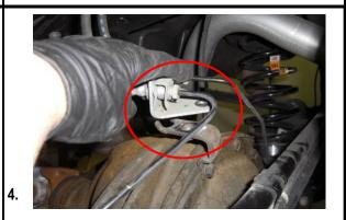
Using a 13mm socket, remove the brake line support bracket bolt.
