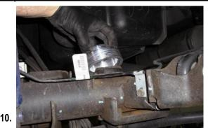
Slowly lower the axle and remove the rear coils and isolator pads. Place the ReadyLift 1.5" spacer on top of the axle
