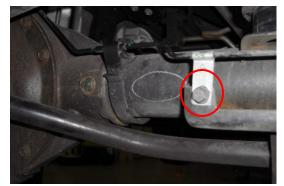
Unbolt the passenger side hard brake line support bracket bolt.
