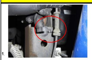
Remove the rear wheels. Unhook the ABS line located at the upper trailing arm mount on both sides.
