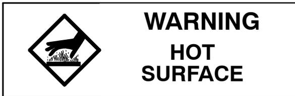
Severe burns can occur if unprotected skin comes in contact with molten adhesive or hot application system parts.
