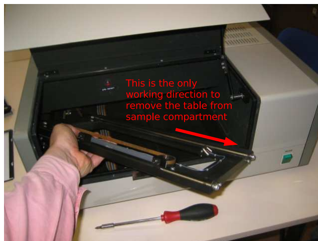
Figure 6.9: Removing the table from sample compartment
