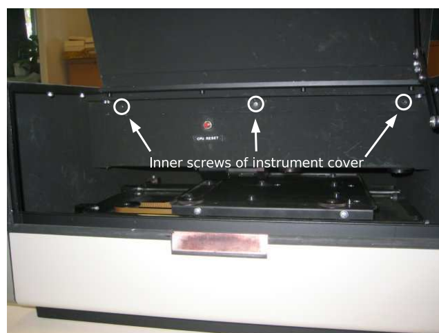
Figure 5.1: Instrument cover screws in the sample compartment
