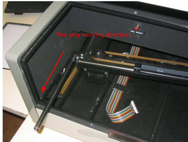
Figure 6.6: How to pull out the shaft
