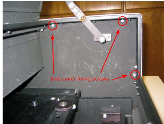
Figure 5.2: Side cover pushing screws in the sample compartment
