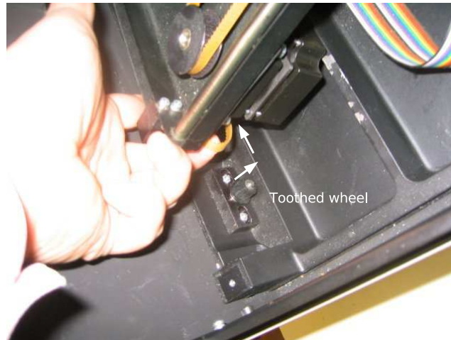
Figure 6.7: Toothed belt removing
