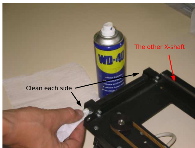
Figure 6.12: Cleaning Y pillow and the other X shaft
