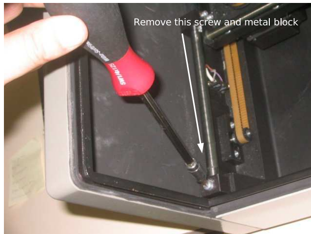
Figure 6.4: Removing table shaft holder
