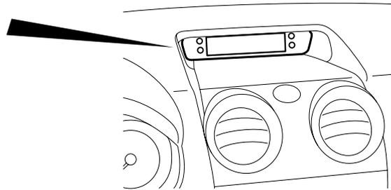
The multi-centre display to provide vehicle information in the text form has been equipped on the centre console as standard. The multi-centre display has the following functions:
