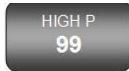
Figure 35 – Setting the High Pressure Alarm Limit
