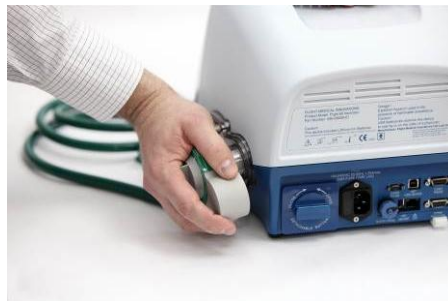
Figure 17 - Air/Oxygen Entrainment Mixer Installation
