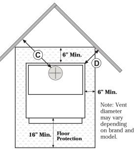
Measure front, rear and side hearth pad clearances from edges of the stove top. Floor protection must be non-combustible and at least .018" thick (26 gauge). Minimum hearth pad sizes: **Model 1250** - 36" Wide x 37" Depth **Model 1750** - 36" Wide x 45 1/2" Depth For all installation and clearance information please consult the Owner's Manual or visit www.avalonfirestyles.com.
