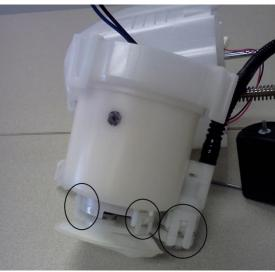
4. Lubricate the new o-ring with fuel or suitable lubricant that is safe for use with automotive fuel systems, and install on the filter inlet that is inside the fuel filter. Use of pliers may be necessary to install o-ring in place due to the inlet's location. Be sure not to damage the o-ring during this process. Re-lubricate the o-ring at this time.
