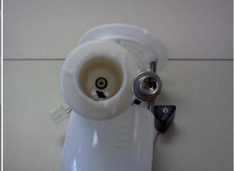
5. Lubricate the inside of the fuel pump outlet and install the pump into the fuel filter. Take care not to damage the oring during installation. There will be a noticeable and positive engagement as the pump seats into the filter housing. When properly installed, the bottom of the fuel pump will be flush with the bottom of the fuel filter.
