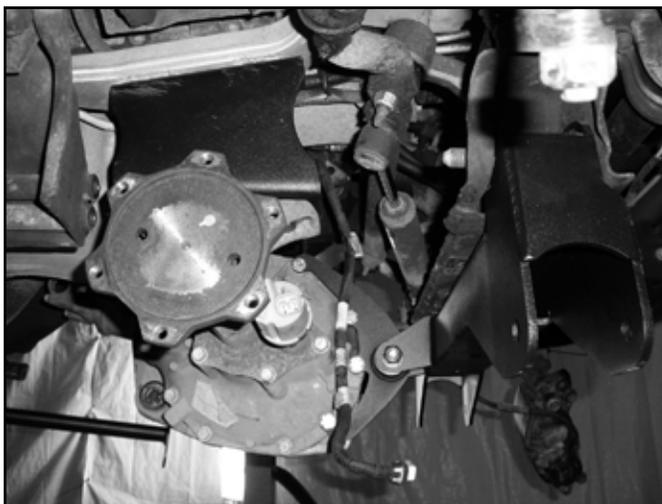
42. Install the new provided bump stops (M02096RB) on the new rear crossmember (02191) with 3/8" hex nuts, flat and lock washers (BP 539). Tighten hardware securely (Fig 24).
