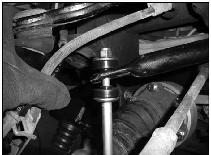
67. Narrow Track Knuckle Kits Only: Reconnect the original brake hose bracket to the upper control arm with the original bolt. Torque to 10 ft-lbs. Attach the second original brake hose bracket to the new "L" bracket install on the knuckle at the upper ball joint with a provided 1/4" x 3/4" bolt, nut and washers (BP 572). Torque to 10 ft-lbs.
