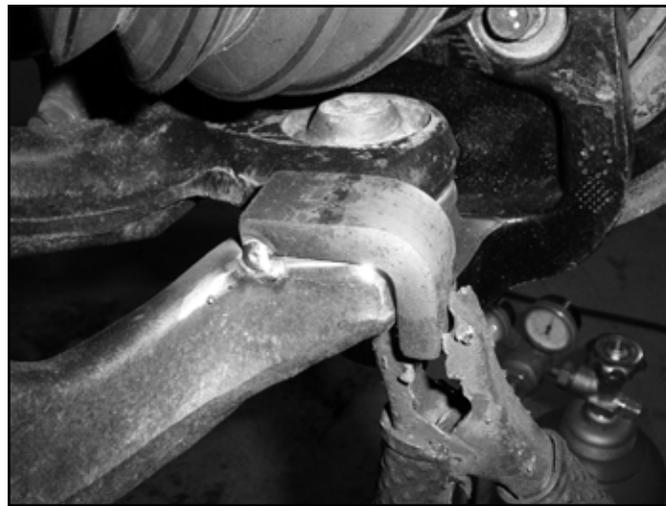
62. Install the brake rotor on the hub. Install the brake calipers on the knuckles with the original bolts. Apply Loctite to the bolt threads and torque the bolts to 125 ft-lbs. Be sure the brake hose is running under the upper control arm and behind the steering knuckle.
