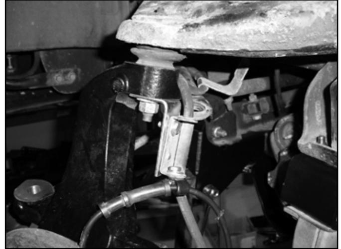
69. Remove the factory clamp and boot from the front driveshaft. Locate the driveshaft boot extension and o-rings. Install the o-rings into the appropriately sized grooves in the extension. Apply grease to the o-rings and slide the extension over the driveshaft with the large diameter first until o-ring snaps over the factory boot lip. (Fig 42)
