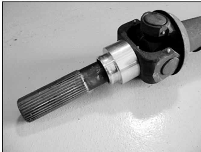
70. Slide the driveshaft into the transfer case and reattach it to the differential with the original clamps/bolts. Torque bolts to 19 ft-lbs.
