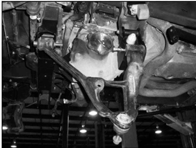
49. Go back and torque the four differential bolts to 90 ft-lbs. Torque the factory control arm pocket bolts to 125 ft-lbs. DO NOT tighten the new control arm bolts at this time. This will be done at the end of the installation.
