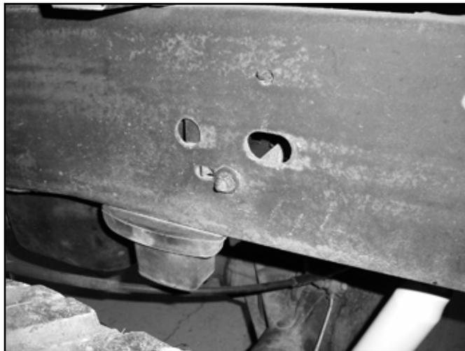
5. Support the center of the axle with a hydraulic jack. Remove the factory shocks from the axle and frame. Save hardware and discard shocks.
