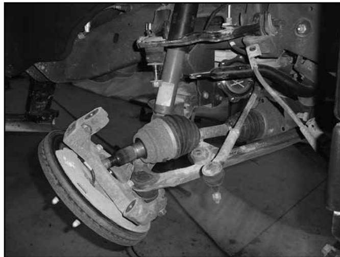
20. Remove the lower ball joint nut and thread back on by hand one or two turns. Strike the knuckle near the ball joint to release the taper. Remove the ball joint nut and remove the knuckle from the lower control arm. Save the lower ball joint nut and set the knuckle/hub assembly aside.
