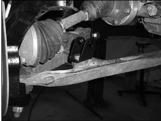
74. Locate the new front sway bar links (911109), small hourglass bushings (SB35BK) and 0.750" OD x 1.575" long sleeves (54587). Install the bushings and sleeves into the eyes of the links. Install the links into the new brackets on the lower control arms with 9/16" x 2-3/4" bolts, nuts and washers (BP 569). Run the bolts from front to rear and leave hardware loose (Fig 43b).
