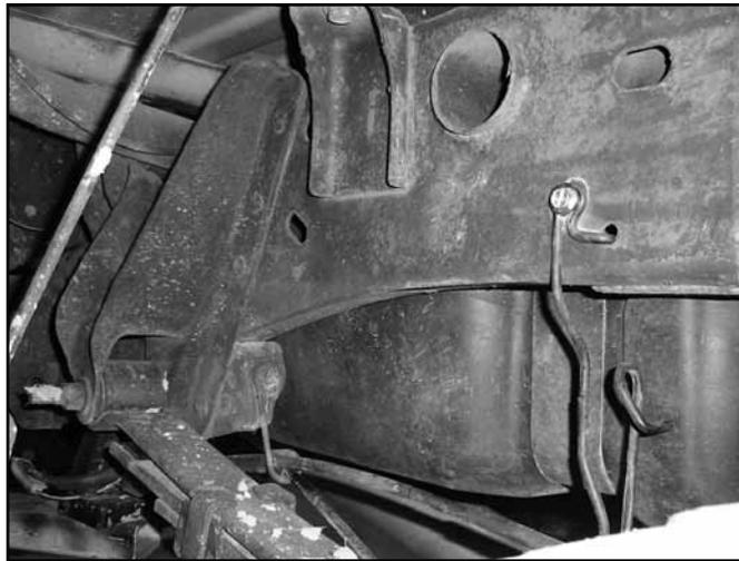
4. Disconnect the factory brake line bracket attached driver's side frame rail. The nut is accessed on the outside of the frame (Fig 47).
