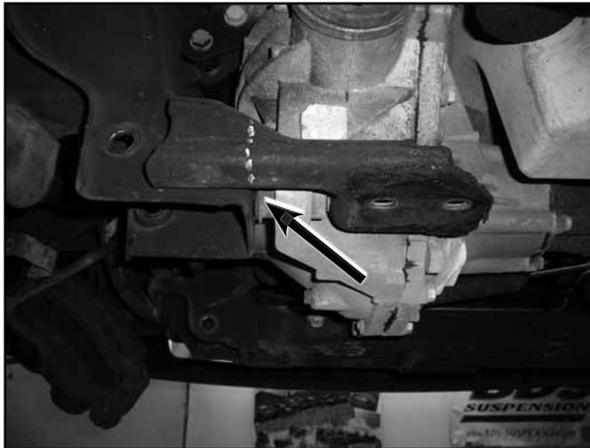
30. Support the front differential with an appropriate jack. Remove the differential mounting hardware and lower the differential from the vehicle and set aside. Save hardware.
