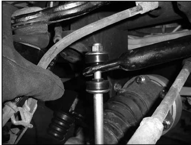
76. Attach the tie rod ends to the knuckles. Fasten with the original nuts and torque to 37 ft-lbs.
