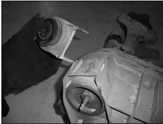
36. Install the provided large bushings (3624RB) and 0.750" OD x 2.950" long sleeve (15) into the eye of the new driver's side differential bracket (01185).
