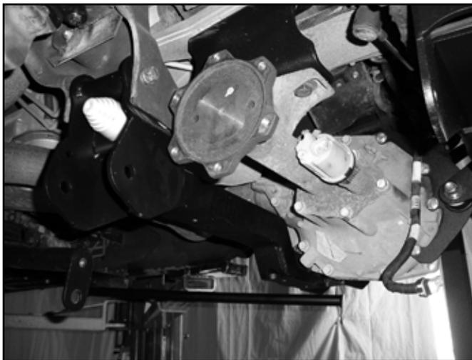
44. Fasten the differential to the new mount in the rear crossmember with the original rear differential bolt/nut. Run the bolt from the outside in.
