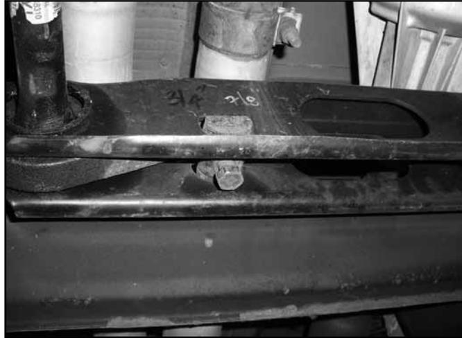
4. Unload the torsion bars but do not remove. Save adjuster bolt/retainer block.
