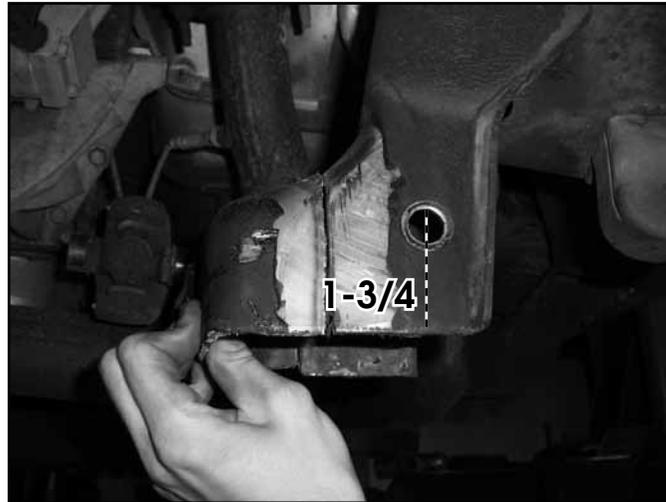
32. Using a reciprocating saw (recommended), hack saw or cut-off wheel, cut the pocket along cut lines.
