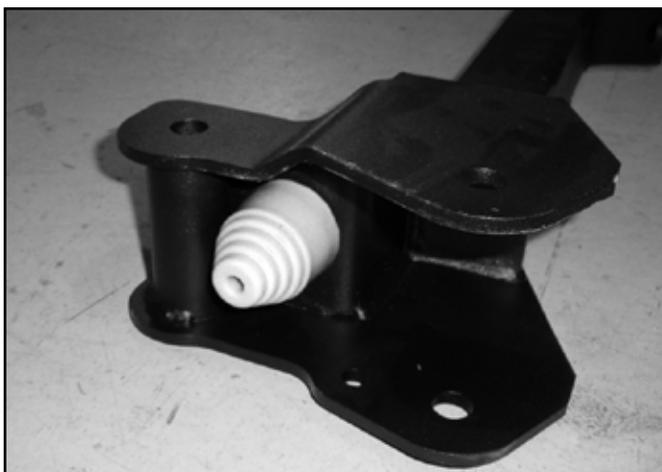
43. Install the rear crossmember in the rear lower control arm pockets so that the differential mount lines up with the differential (Fig 25) Fasten the crossmember with the original lower control arm hardware. Run the bolts from front to rear. Leave hardware loose.
