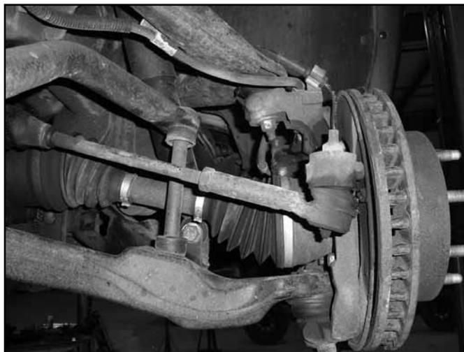
12. Disconnect the ABS brake wire from the connector at the top of the frame (Fig 5) Remove the wire from the plastic retainers on the frame and upper control arm (Fig 6).
