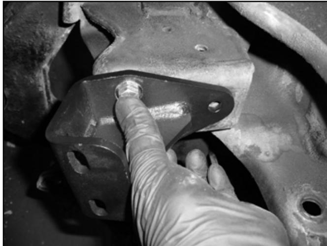
47. With the holes drilled, attach the new brackets to the frame with 3/8" x 1-1/4" bolts, nuts and 3/8" washers (BP 572). The two outer bolts should be all the way to the outer edge of the slots in the brackets (bracket push inward toward frame as far as possible). Torque bolts to 30 ft-lbs. Install the factory bump stop on the new brackets with the original mounting nut. Install the bump stop so it is offset toward the rear of the vehicle (Fig 28). Tighten bump stop hardware securely.
