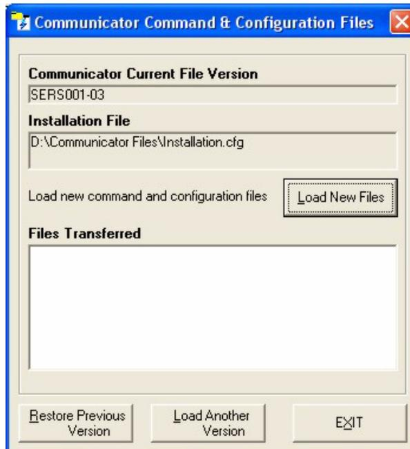
**Figure 75 - Communicator Software Installation - Command and Configuration Files**
