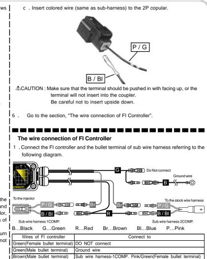
2 . Connect the coupler of sub wire harness 1COMP. to the injector.
