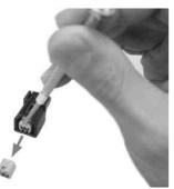
b.Pull out the wires individually from the coupler with a pick while pulling up the inner hook fixing the terminal of the stock coupler. At this time, you do not have to remove the retainer on wire side and rubber seal.
