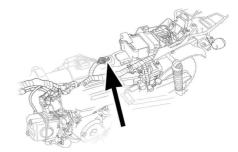
5 . Disconnect the 2P coupler of stock wire harness connecting the injector.
