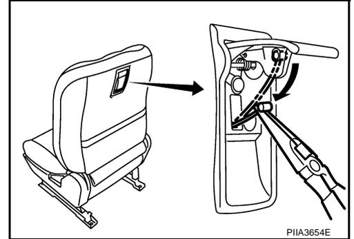
2. Disconnect the harness connector, and then remove seatback switch.
