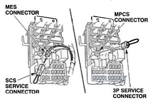
Use the 2P MES connector, along with the SCS service connector (T/N 07PAZ-0010100), to clear SRS DTCs (see section 23 of the 2002 CR-V Service Manual).
