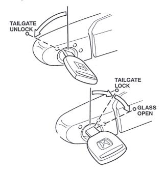
You can open the hatch glass either with the remote transmitter or by pressing the hatch glass release button on the driver's door. You can also open the hatch glass by inserting the key into the lock and turning it *clockwise* to the release position. Note this also locks the tailgate.
