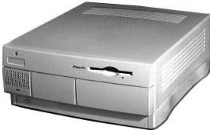
Like the other Macs it resembles the PPC 7500 does have some very impressive features inside: eight DIMM slots for up to 512 Megs of RAM, two SCSI DMA buses supporting up to eight SCSI devices, three PCI expansion slots, one Digital Audio Video (DAV) slot, built-in AUI and 10Base-T Ethernet, video-in support via external ports, two GeoPort Serial ports, built-in CD-ROM, and CD quality stereo sound in and out. What it lacks in processor power makes it a very likely candidate for upgrading.
