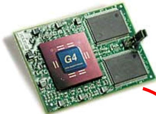
**Here's a ZIF G4 Upgrade, above, as it appears ready to go into a G3 and here is the same upgrade below, being installed onto a carrier to be put into an early PowerPC.**
