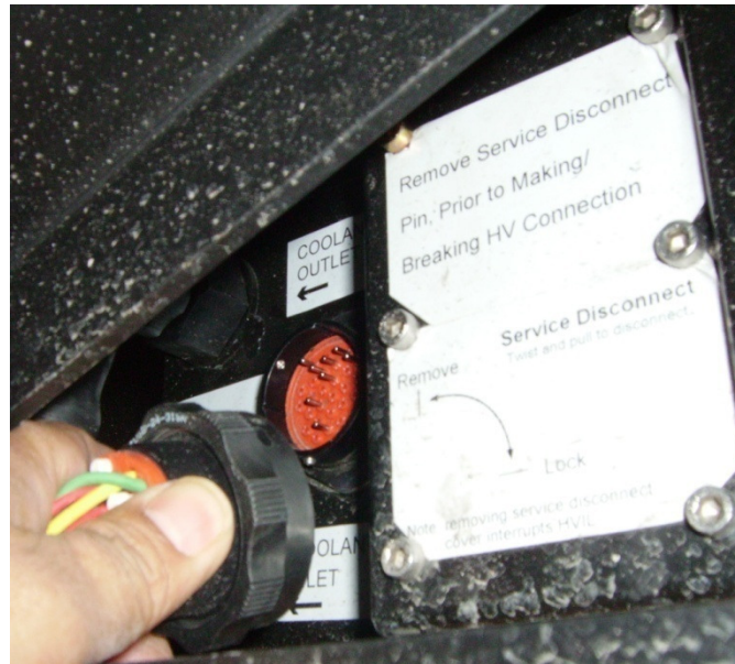
Figure 2: Removing Low Voltage Connector from High Voltage Battery Pack
