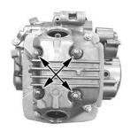
Tighten the cylinder head cover nuts first, and then the cylinder head cover bolts. Tighten both of them in several steps diagonally. Specified torque: for cylinder head cover nuts  $:27 \text{ N} \cdot \text{m} (2.8 \text{ kgf} \cdot \text{m})$ for cylinder head cover bolts  $:12 \text{ N} \cdot \text{m} (1.2 \text{ kgf} \cdot \text{m})$
