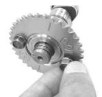
h. Remove the loosened two bolts on the cam sprocket. Then fix the cam sprocket to a cam shaft of the kit, and tighten the two cam sprocket bolts temporarily.
