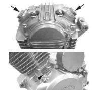
a. Remove two tappet hole caps, a crank shaft hole cap, and a timing hole cap.
