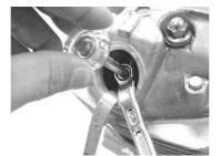
If you need to adjust the clearance, loosen the nut and tighten the adjusting screw.
