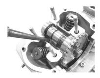
d. Fill up the oil pool in the cam with fresh engine oil.
