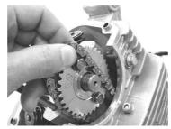
c. After checking that the cam chain is fit in the timing sprocket of the crank shaft, fix the cam chain to the cam sprocket.
