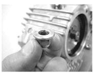
Apply engine oil to the threaded part and the seating face.
