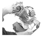
d. Holding the flywheel tightly, loosen two cam sprocket bolts.
