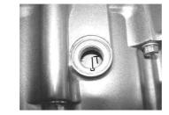
a. Check that the "T" mark on the flywheel is aligned with the alignment mark on the crankcase cover.
