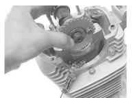
g. Detach the cam chain from the cam sprocket to<br/>remove it.b. After applying fresh engine oil to the bearings,<br/>install the cam shaft so that the engraved lines
