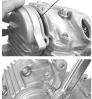
c. Fix a gasket of the kit to the cam sprocket cover, and install the cover to the cylinder head. Install and tighten two bolts. Specified torque:10 N • m (1.0 kgf • m)
