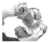
g. Holding the flywheel tight, fully tighten the temporarily-tightened two cam sprocket bolts. Specified torque:12 N • m (1.2 kgf • m)
