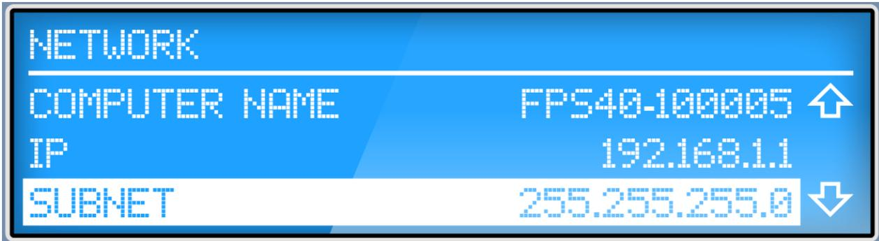
The R&S FPS is equipped with a miniature display on the front panel that provides basic information and allows for very basic instrument configuration (such as changing the IP address). For details see [chapter 4, "Miniature Display"](#), on page 37.
