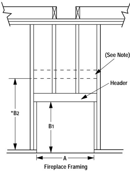
\*Note: When Framing With 6" Studs Header Must Be 17" (432mm) Higher. Use Security Chimney's OR15 Offset/Return Elbow To Recess The Chimney Back 2 1/2" (64mm). Flat Frame Down To A False Header At (B1). Maintain Required Clearance To Chimney At All Times.
