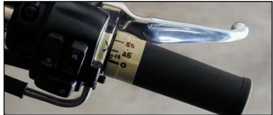
The throttle position marks will correspond roughly with the MAP readings in the table provided in this section.
