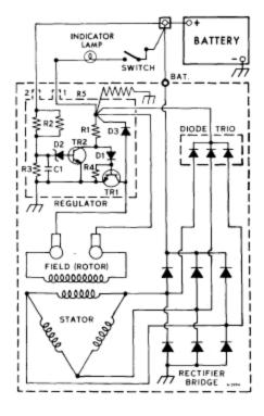
Figure 23—Schematic Diagram of Generating System (Typical)
