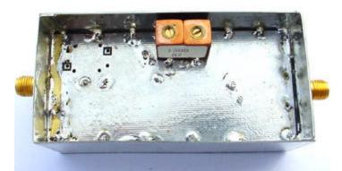
Bottom of LNA view where the 2 stage helical filter is, the holes to the left of it are for another filter which I have elected not to fit at this time.
