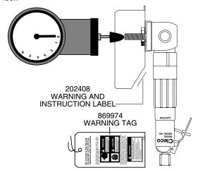
The speed rating, warning tags and warning labels should be maintained or replaced for legibility in the event of damage. Speed rating, warning tags, and warning labels are available from the manufacturer.
