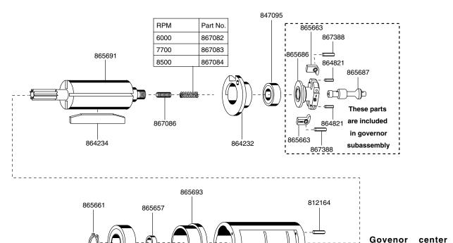
865687, govenor weights No. 865663 and Pins No. 867388 should be checked periodically for wear and replaced when necessary.
