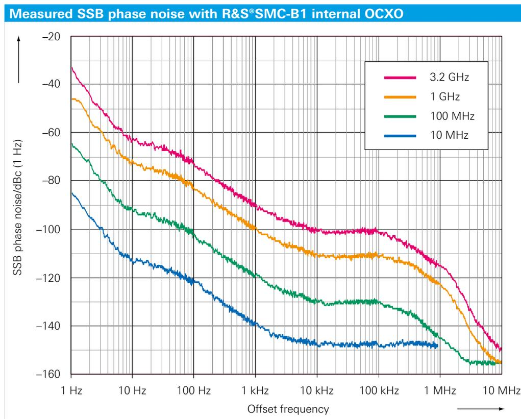
Measured SSB phase noise at 20 kHz offset versus frequency
