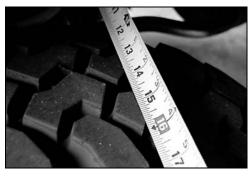
**HINT**: For example, measure from the edge of a tire tread lug to the outboard side of the chassis, then repeat the measurement on the other side of vehicle using exact same points.
