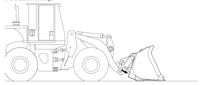
4) After the KAT Master Hitch is fully seated, extend the lock pins, engaging the attachment.
