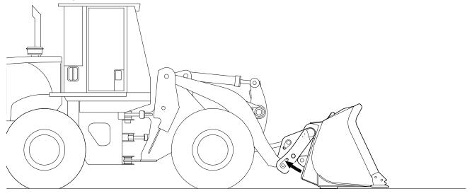
5) Once the KAT Master Hitch has cleared the attachment, position the machine to engage another attachment.
