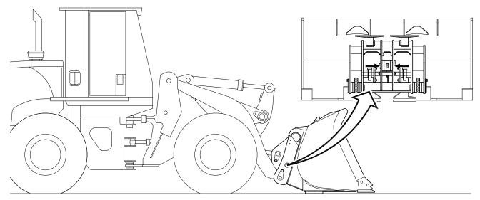
4) After the bottom end of the KAT Master Hitch is disengaged, lower the machines lift arm/boom to free the top end of the hitch.
