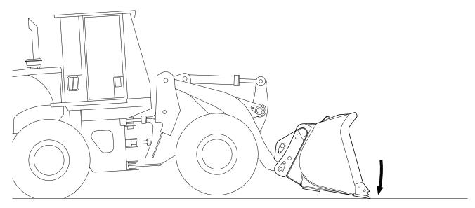
8) After the visual inspection and secure engagement test has been successfully completed, and proper attachment to the KAT Master Hitch has been confirmed, operate the machine as required.
