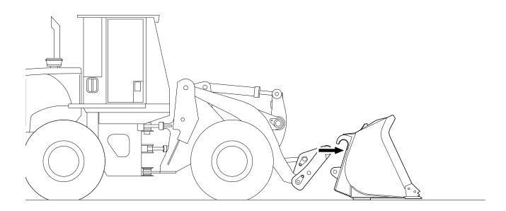
3) When the top bar of the KAT Master Hitch is fully inserted in the top hooks of the attachment slowly tilt the Master Hitch back to rotate the bottom of the Master Hitch into the lower portion of the attachment lugs.
