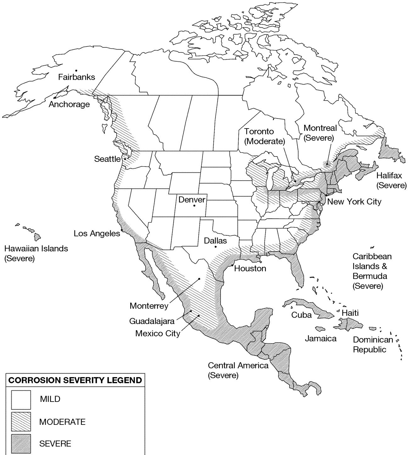
North America Corrosion Severity Map Figure 2 (Sheet 1)
