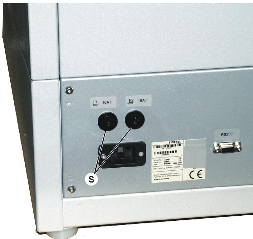
1. Unlock the cover of the fuse holder (**S**) with a screwdriver (press the cover slightly and turn it counterclockwise).
