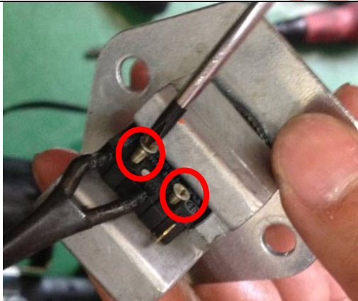
STEP 7: Remove 2 screws fixing the Micro switch for lifting with screwdriver, and then you can remove and replace the micro switch.
