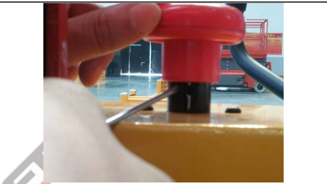
STEP 2: Use a small screwdriver to insert the hole and remove the screw
