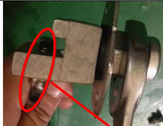
STEP 8: Dismantle the screw and the seat of micro switch with 2 wrenches, one is for holding.
