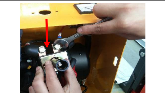
STEP 5: Pull down the emergency button, and remove 2 screws fixing the cable with 12mm wrench.
