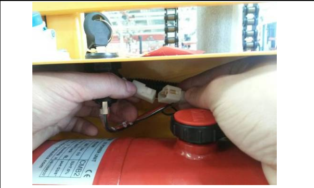
STEP 2: Dismantle the connector, now you can remove it.
