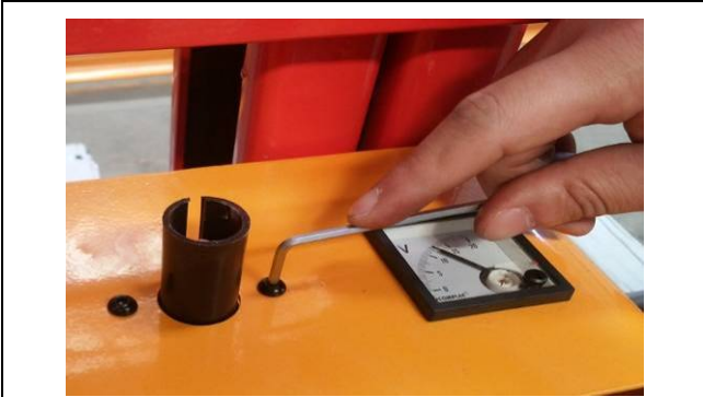
STEP 4: Remove 2 screws beside the button with 3mm Allen wrench
