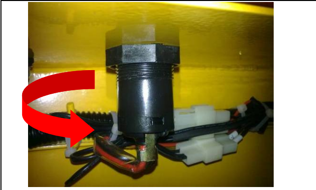
STEP 1: Turn counter-clockwise the key switch with wrench.
