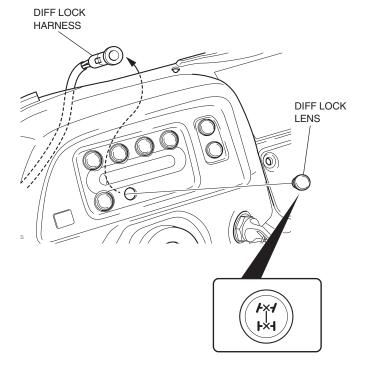
11. Cut out the instrument panel as shown. Remove any burrs from the edges of the hole.
