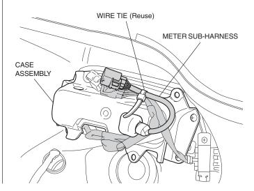
21. Reinstall the instrument panel. Connect the meter sub-harness to the vehicle's harness. Reconnect all previously disconnected connectors.
