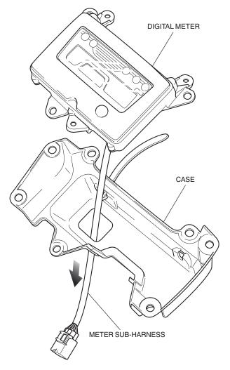
9. Assemble the digital meter as shown.
