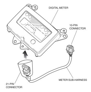
8. Pass the meter sub-harness through the hole of the case.
