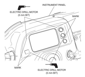
18. Install the meter cover as shown.
