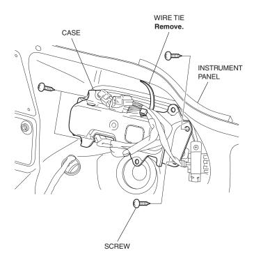
6. Cut out the case as shown. Remove any burrs from the edges of the hole.
