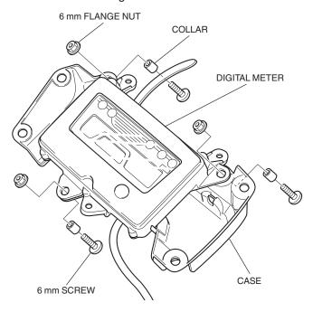
10. Remove the diff lock lens and harness as shown.
