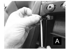
**Caution:** Over tightening may cause door to not open freely and fatigue hardware. Repeat for rear door on 4 seat models.
