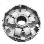
Be careful that no oil or grease will stain the movable drive face or spacer. Be sure to degrease the face or spacer whenever stained with oil or grease.
