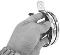
4 . Attach the silencer band to the stay with an 8x20 flange bolt and M8 flange nut, sandwiching the stay.
