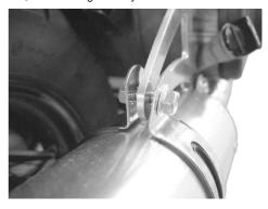
5 Fit a 6x25 flange bolt into the collar attached to the stay, and install for now the exhaust pipe on the muffler COMP. with an M6 flange nut.
