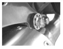
6 . Tighten the exhaust pipe nut to the specified torque.
