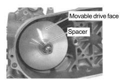
(Install supplied six weight rollers.)
