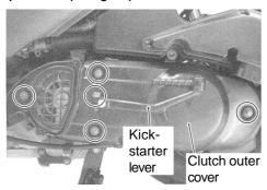
Unscrew a clutch cover bolt to remove a clutch cover.
