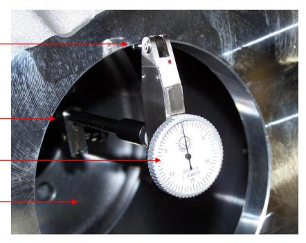
Make sure the indicator has adequate travel in both directions and will be in constant contact with the bore register during the entire 360 degrees of rotation so that you will obtain accurate readings. It is not necessary to begin at a certain position on the bore, any point will work. Mark the point where you begin on the bellhousing with a hash mark using chalk or a marker as a reference.
