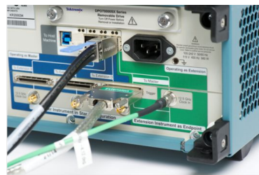
UltraSync connection on instrument with Extension role
