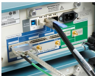
UltraSync connection on instrument with Master role
