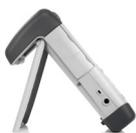
When laid out flat for operation from above, the R&S ZVH is still tilted slightly because of the grip on its top. This position provides the optimum viewing angle for the display.
