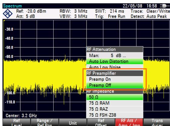
The magnitude of amplification depends on the reference level. This coupling to the reference level makes sure that the dynamic range is at an optimum.
