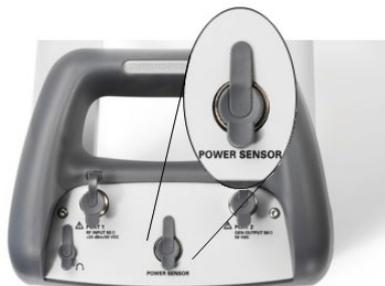
The connector is configured especially for power sensors. It is used for both the power supply and data transfer via the power sensor interface.
