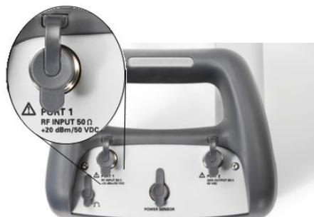
Connect a cable or DUT to the RF input with an N connector. Use a cable to connect the DUT to the R&S ZVH, if necessary.
