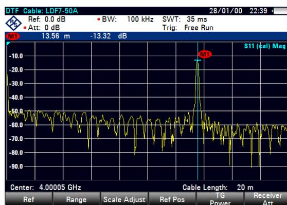
A blue vertical line represents the position of the marker on the horizontal axis (e.g. the frequency).
