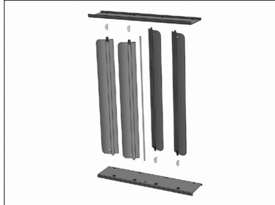
Figure 4.2 – Vertical Louver to Unit Installation
