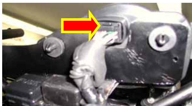
Figure 2: unplugging the on board dash connector
