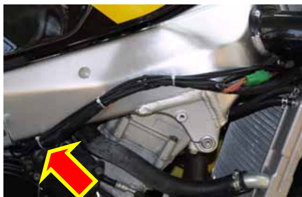
Figure 12: Wiring installation: run the wiring along the chassis
