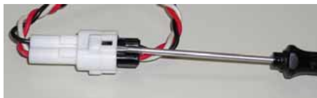
Figure 6: How to unplug a connector
