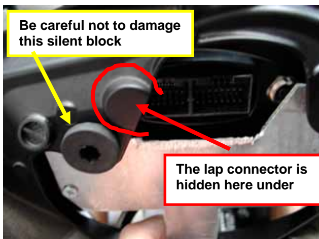
Figure 7: the part of the chassis to milled.
