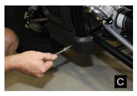
**Step 4:** Install bumper by aligning upper tabs with L-brackets, secure with supplied hardware. Then secure lower bumper tubes with supplied hardware utilizing holes where screws from **(Step 3)** were previously removed. **(See Figure D & E)**
