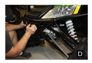
**Step 5:** Go through and tighten all hardware (you can reference service manual for torque specs). When all hardware is secure insert tube end caps by pressing into place. (See Figure F)
