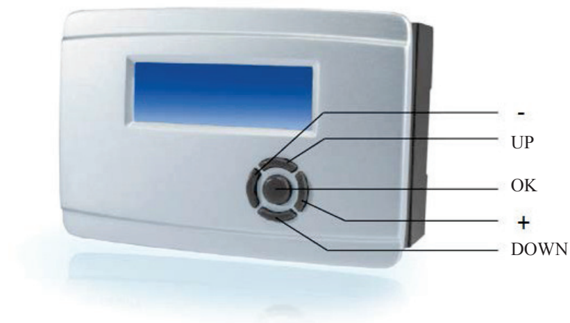
Fig. 1.2: The control elements
