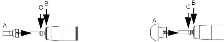
3. Gently push and twist the eartip (A) onto the probe tip, until it rests firmly against the base of the probe (B). Make sure that the eartip covers the collar (C) of the probe tip.
