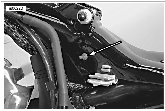
Figure 5. Converter Module Mounting Tab (2008 and Earlier)
