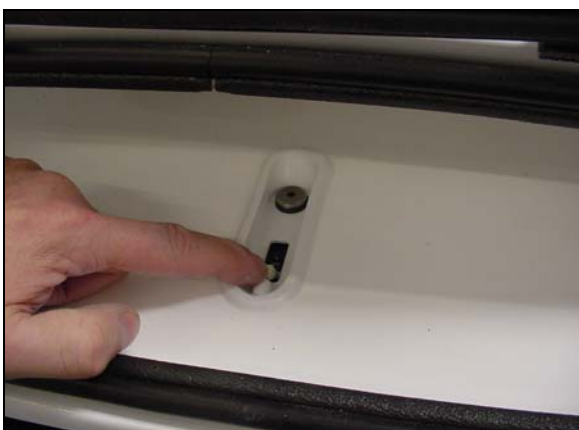
Power breaker in glove box
