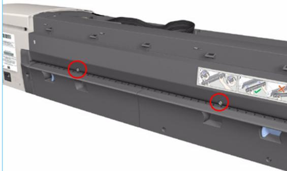
5. Remove 2 T-10 screws that secure the Center Cover from the rear.
