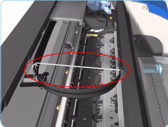
3. Release the Tubes from the retaining clips in the Center Cover.
