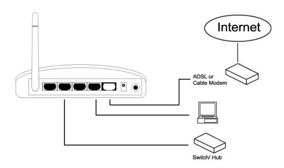
Connect the power adapter to the wall socket, and then connect it to the "12V" socket on the back panel of the router.
