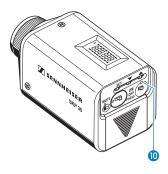
The red LED (1) and the 8-segment bargraph on the display provide information on the (remaining) battery capacity.
