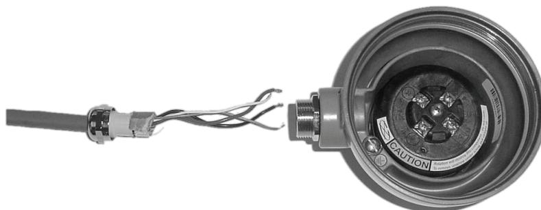
5. Insert the wires through the gland body and assemble the gland by tightening the gland nut. If desired, leave sufficient wire length inside the core processor housing to allow the housing to rotate without damaging the wires.
