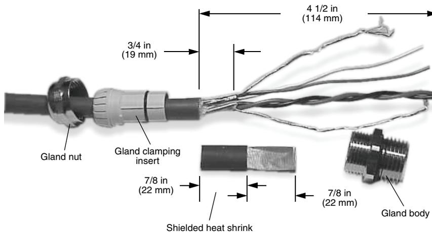
4. For connection at the core processor housing, prepare shielded cable as follows (for armored cable, omit steps d, e, f, and g):
