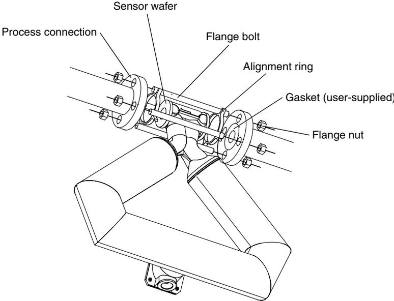
Figure 13 Tightening the sensor alignment rings
