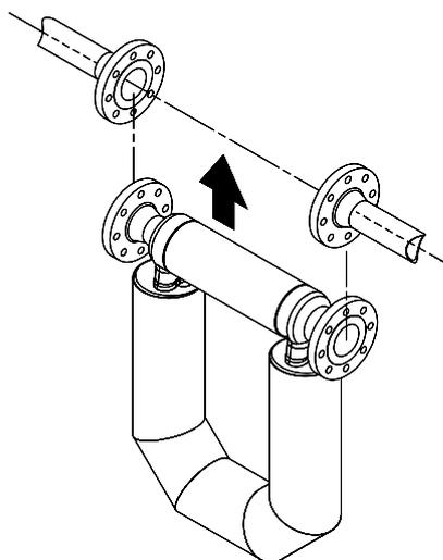
**Figure 8 Optional mounting for CMF010 sensors**
