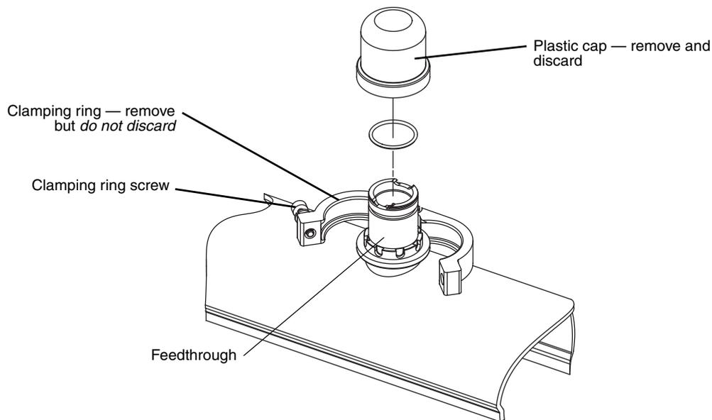
**Figure 10** Mounting the temperature extender onto the sensor
