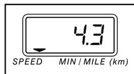
measured in *minutes per mile*). The display will alternate between one number and the other every seven seconds, as shown by the arrows in the display. Note: When the SPEED buttons are pressed, the display will show the current speed setting.
