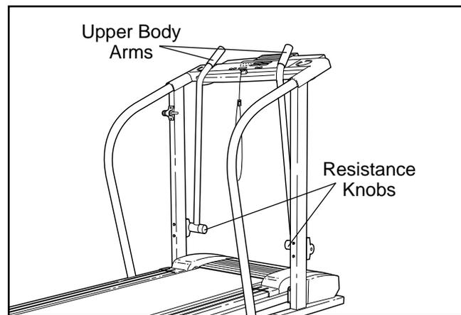
To vary the intensity of your upper body exercise, the resistance of the upper body arms can be adjusted. To increase the resistance, turn the resistance knobs clockwise; to decrease the resistance, turn the knobs counterclockwise.
