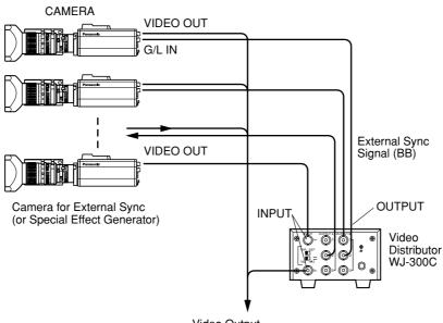
Video Output To Special Effect Generator or Monitoring System
