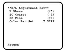
[ADJUSTMENT with RCU (RCB, Hybrid control panel)] Use the subcarrier phase coarse adjustment control and subcarrier phase fine control.
