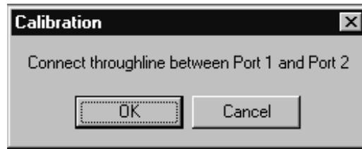
**Step 8.** Press "OK" to complete the S Parameters calibration (below).
