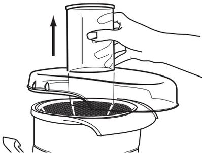
5. Place fingers under the rim of the stainless steel blade and filtering basket and lift out – figure 11.
