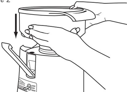
3. Position the stainless steel blade and filtering basket onto the motor drive shaft and push down until firmly in place – figure 3.
